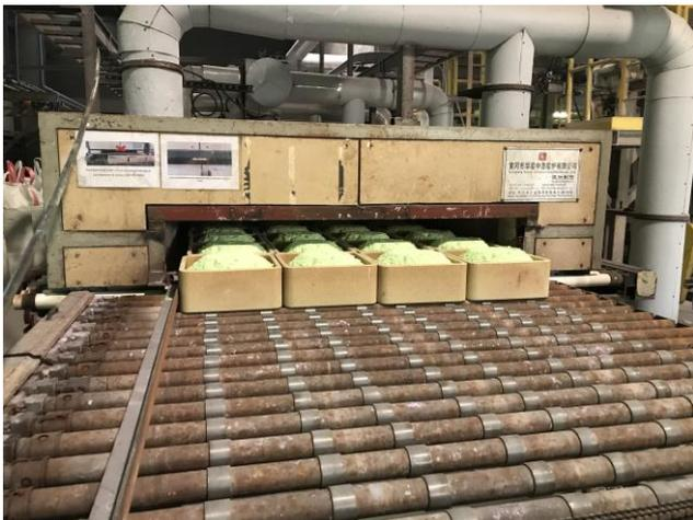
*Pr oxalate feed into Tunnel Furnace for calcination*
