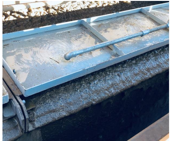
Cleaner 2 at Mt Weld with new froth washing, Cleaner free flowing froth
